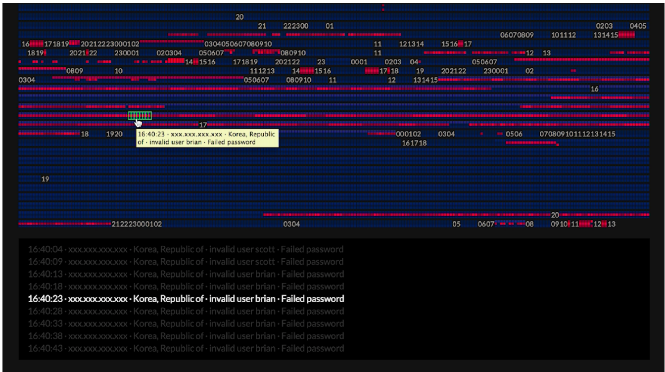
Fig. 4: Video showing the main interactive techniques currently implemented for the Pixel Carpet: highlighting of identical records, tool tips and clear text display, and filtering/removal on click. The numbers in the Carpet refer to the hours from the time stamp. Two consecutive numbers mean that all records in between got filtered away. (Data from ssh log file, IP addresses replaced for publication).
